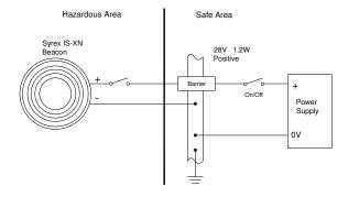
Fig 3 Using a single channel barrier.
